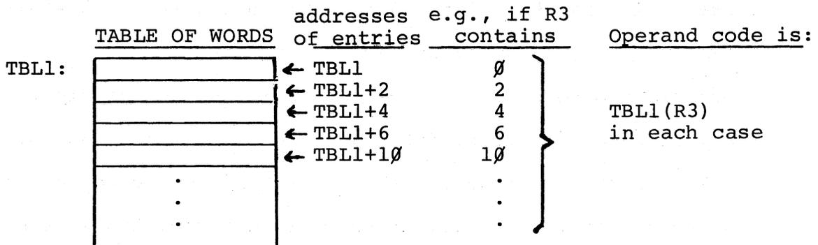
When deferred Index Mode is specified (e.g., @TBL1(R3)), the calculated address contains a pointer to the data, rather than the data itself. Byte tables are discussed in Section 1.8.
