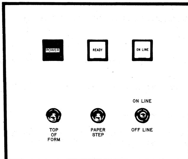
Figure 2-5. Line Printer Control Panel
