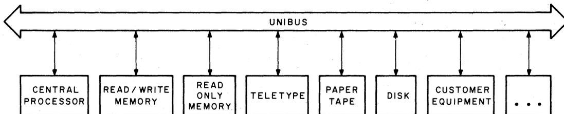
Figure 1-3 PDP-11 System Unibus Block Diagram
