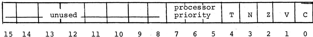
Figure 1-2. Processor Status Register
