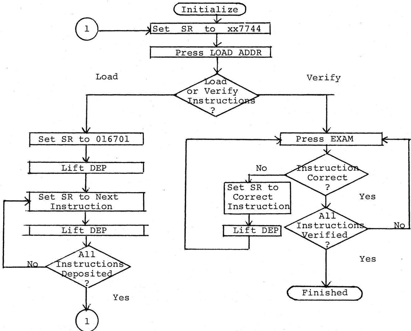
Figure 6-2. Loading and Verifying the Bootstrap Loader
