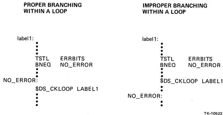
Figure 3-7 Proper and Improper Branching Within Loops
