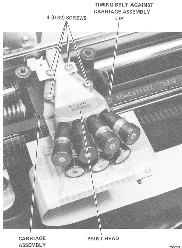
Figure 20 Print Head Removal
